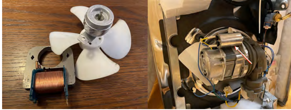
FIG. xi An induction motor for a small fan (left) and an induction motor for a dishwasher (right), with capacitor indicated by the arrow.
