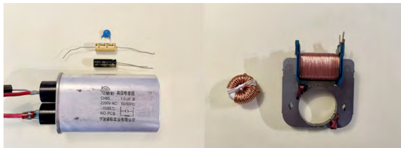
FIG. ix Capacitors (left) ranging from baby (top) to momma (bottom); inductors (right).
